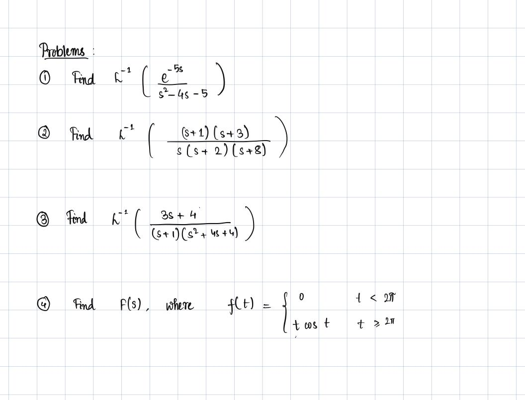
$$\begin{array}{c} \widehat{0} \ F(s) = \underbrace{e^{-5s}}_{s^2 - 4s - 5} = \underbrace{e^{-5s}}_{s^2 - 5s + s - 5} = \underbrace{e^{-5s}}_{s(s - 5) + (s - 5)} \\ = \underbrace{e^{-5s}}_{(s + 1)(s - 5)} \\ \underbrace{e^{-5s}}_{(s + 1)(s - 5)} = e^{-5s} \left( \frac{A}{s + 1} + \frac{B}{s - 5} \right) \\ A + B = O \\ -5A + B = 1 \\ (A = -V_6) \\ \underbrace{e^{-5s}}_{(s + 1)(s - 5)} = e^{-5s} \left( \frac{(-V_6)}{(s + 1)} + \frac{V_6}{(s - 5)} \right) \\ \end{array}$$
