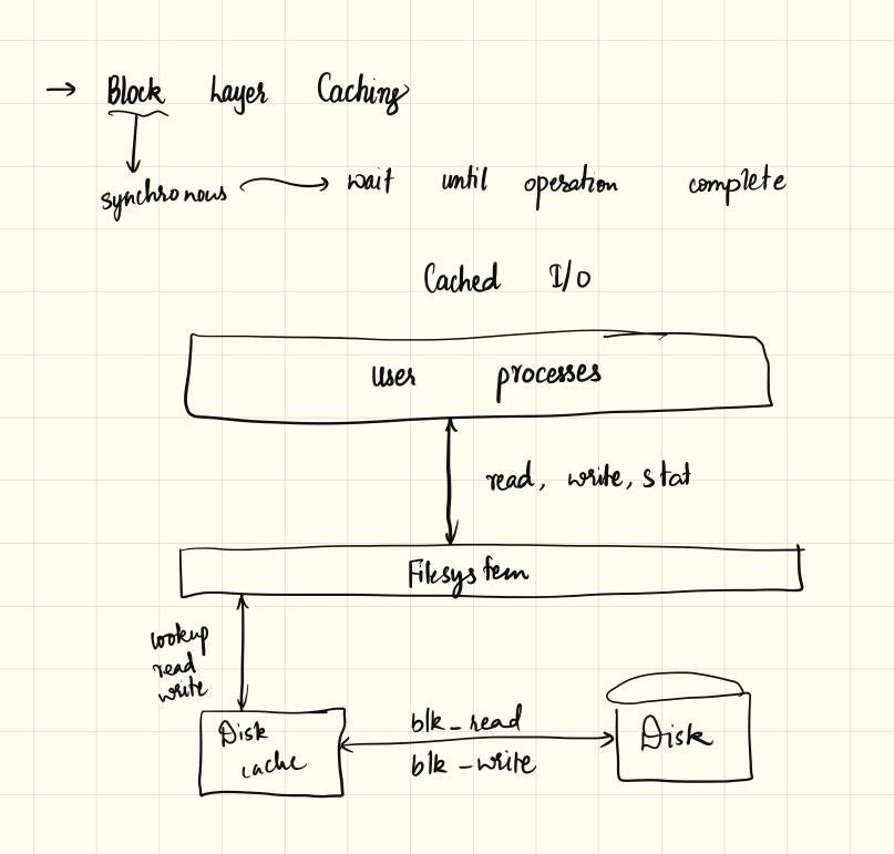
Lookup memory cache using block number as the kuy For data caching, block address mapping is required before Data Metadata using the cache > works fine for metadata as they are addressed using block #
